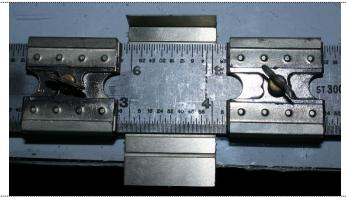
With one clamp in place on the rulers slide the work piece between the rulers then slide the other clamp in place, line up the etched fold line with the edge of the rulers, then tighten the screws.
