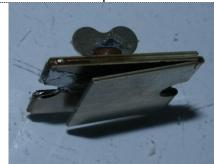
Fold the spring 180° <u>toward</u> the etched line This forms the spring plate
