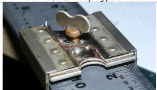
Insert the 2 halves, use rulers to force the spring up and solder the sections together. Remember to remove the screw!!
