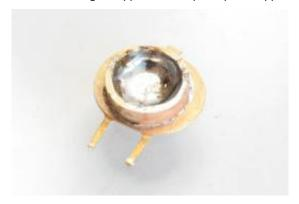
Cut a 2mm length of the 3/16 tube and solder it to the back of the lid
