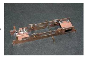
Remove the chassis spacing jigs by breaking the soldered joins.
