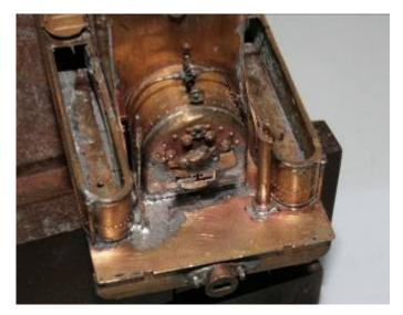
Now guess the approximate position of the thread and drill a 1.0mm hole in the cab floor above this. Dismantle the body from the chassis. Mount the brake handle (G) into the hole and solder it in place from under the floor.
