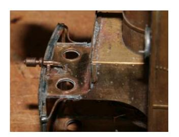
Trim the whistle pipe and check the fit of the whistle, the bracket should rest just under the roof. When you are happy with the fit clean and tin the whistle bracket then place in position and solder.
