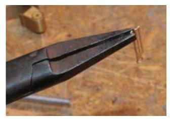
Fold the mounting bracket down 90° and reinforce the fold with a good fillet of solder.
