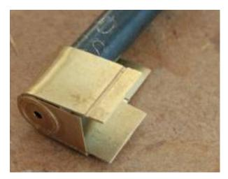
Using the shank of a 4mm drill as a former gently bend the cylinder wrapper, work it around until the half etch lines on the ends of the cylinder wrapper clip into the holes in the side frames.
