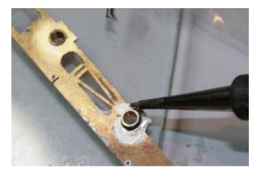
Lay the side frame down onto a flat surface to ensure the bearings remain square during soldering
