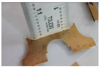
Fold the sides back 90°, be careful not to flatten the rivet details, hold the inside piece in a pair of long nose pliers right against the fold line and then gently eased the side up by flattening it on to the bench
