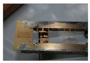
Fold the springs up 90°behind the side tanks and reinforce the folds with a fillet of solder. Run a fillet of solder along the inside of the cab assembly.
