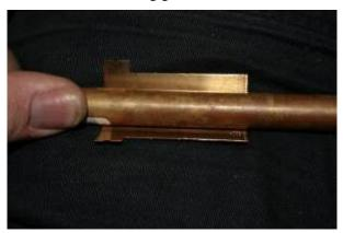
With a sharp knife cut along the guide line and remove the extra piece from each side of the boiler (5). Punch the rivet details along the back edge and around the washout plug. Progressively roll the boiler using a round bar then the shank then a 10mm drill to form the boiler into a "U" shape, check the shape by fitting into the cab front - sand box and onto the backhead
