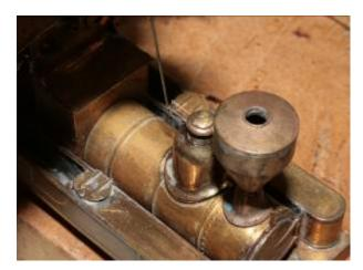
Take the relief spring bracket (53) and solder a 5mm length of  $1/32^{nd}$  tube to each end. Bend each tube end up  $90^{\circ}$ .
