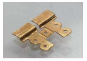
Step 2: Clamp the crosshead at the first fold against something thin, a 6" steel rule which is about 0.5mm thick is good, fold the next section up  $90^{\circ}$  while forcing into the first fold, don't be gentle, these folds need to be  $90^{\circ}$  opposite each other.
