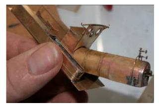
Test fit the boiler by feeding it into the hole in the cab then letting it rest up between the side tanks. File the inside of the cab hole until the boiler fits up and the top is parallel to the side tanks
