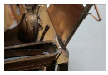
Tack solder the cab rear to the floor inside the cab and check that all the parts are aligned then tack the other side.
