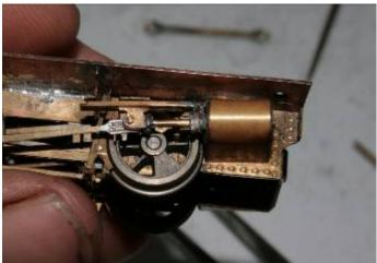
Insert the cylinders into the chassis bend the ends of the cylinder tabs out to retain the cylinder. Check the clearance between the crosshead and the crankpin.
