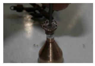
Before removing the funnel base flange from the sprue drill a 1.0mm hole through the centre and a 0.4mm hole in the edge of the flange for the smoke box oiler. Cut the feed web out of the underside of the flange. Clean up the funnel top casting with sand paper.
