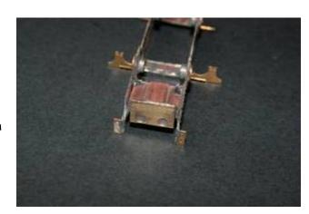
Now we can add the brake hanger pivots. Open out the 0.5mm holes with a broach or the tip of a round file to fit the 0.5mm wire. Place three lengths of wire through the two holes at the top of the frames and one through the hole at the cab end and leave a 5mm overhang out each side of the frame.
