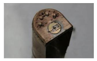
Take the fire box shelf (20) punch the rivets and fold the brackets 90° then solder this to the back head just below the line of rivets. Clean the bottom of the oil can and tin it, then solder the oil can to the shelf.
