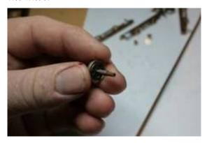
Line up the wheel and half an axle in the jaws of your bench vice and squeeze the part together until the 2mm turned end is pressed home into the wheel
