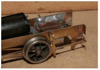
Place the rear hangers, brake rods and crank assembly onto the 0.5mm pivots and align the shoe up against the wheel
