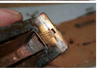
Remove the front plate (16) and from bends in both ends until the plate fits into the gap at the front of the footplate and into the front headstock. Once the shape fits correctly solder it in place from underneath. Give it a wash and file back the end until they are flush with the footplate.
