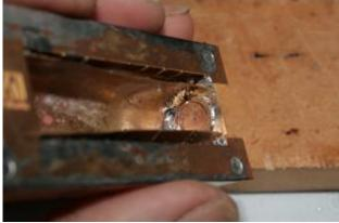
Position the boiler so it lines up with the outer edge of the smoke box front. Solder the boiler in place from the back of the smoke box front inside the boiler.
