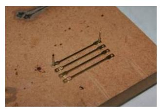
Clear out the holes formed by the half etched lines to 0.3mm and pass a short length of 0.3mm wire through each hole. Add some flux to each wire and heat this should be enough to sweat solder the wire in place. Trim the wires back to represent bolts.
