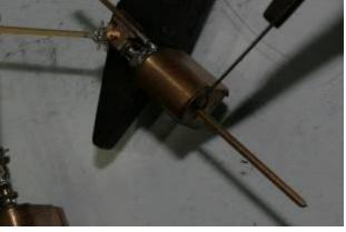
Cut the piston rod to length, mark the rod at both extremes of travel
