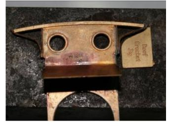
Punch the rivet details on the roof brackets, now bend the roof brackets back 180° then form the roof brackets to shape using the roof bending jig as a guide, don't worry too much about getting this right at present. To form the angle iron edges of the cab, clean up the edges of the laminate and fold the side angles forward 90° to cover the laminated edge. Solder everything in place. Now give it a wash.
