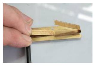
Form the rounded ends of the tanks by working them around the shank of a 5mm drill, the curve around the 5mm drill is a little tight so only go far enough to get the ends to meet. The mating ends are designed to interlace.
