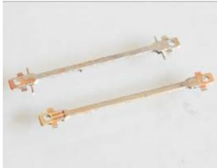
Open out the crankpin holes to fit the Northyard crankpins, these are 1.6mm in diameter. The best tool for this job is a cutting broach.
