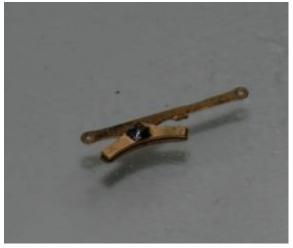
Place the front hangers onto the 0.5mm pivots and align the shoe up against the wheel, now solder the front hangers to the pivots.
