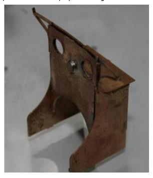
Align the cab front with the rear row of rivets, the sand box sides and the cab side angles should line up to form a close butt joint. File the cab sides and square off the edge of the cab front angle to get the nice flush joint.
