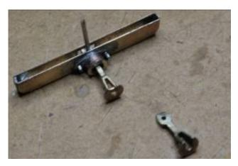
The headstocks are designed to fit either the MMW or NZF couplers, if you desire to fit another type then you will need to modify the headstocks to suit. The simplest means of mounting the coupler is to insert a short length of 1mm rod through the coupler mounting hole inside the headstock this will lock the coupler in but allow it to move around freely, alternately with the MMW coupler you can solder a 0.4mm wire into the slot in the coupler and use this to mount the coupler onto the body.
