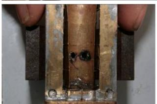
Remove the waste from the steam dome and clean up the bottom surface and tin with solder. Using a fine needle file carefully file a small flat on the back of the dome just in the narrowest point and tin with solder.
