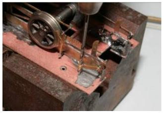
Take the hand brake operating arm (27) and the 14BA screw. From the pivot nut from the flat end of the operating arm by carefully wrapping it around the 14BA bolt. Check the length of the thread, it needs to be 90° to the PCB with the end of the operating arm on the short brake crank adjust as necessary and solder the thread to the mounting PCB.
