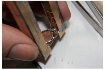
Position this between the side tanks, it should line up with the step in the floor and the rib on the side tanks. Check for square and solder the smoke box front in place from the back.
