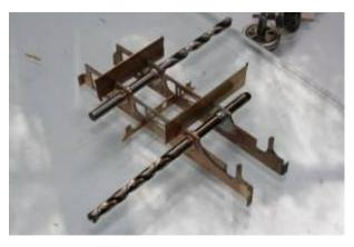
Cut a 3mm long piece of the 0.4mm PCB spacer, solder it to the motion bracket through the holes provided and the other side to the side frames. Now give it a wash.
