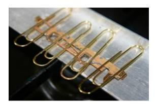
Bend the pieces 180 degrees together and clamp them together. You can use any type of clamps, they just need to be able to stand the heat.
