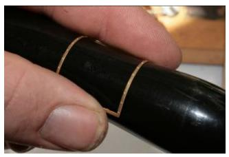
Solder the frame at the corners and make final adjustments to the roof brackets then solder the roof end in place to the side angle of the roof frame. Now give it a wash.
