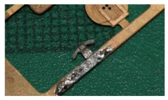
To form washout plate clamp (7) leave it attached to the fret and fold it 180° back on itself then solder it together. Clear the hole through the centre to 0.35mm, remove from the fret, then thread a short length of 0.3mm wire through the clamp and solder it in place. Place the washout plate clamp through the hole in the centre of the wash out plate. Solder it in place from the inside of the boiler
