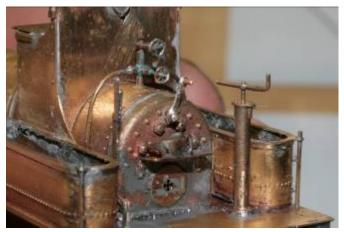
If you want to install the cab mounted whistle, start by drilling a 0.55mm hole through the cab front between the windows
