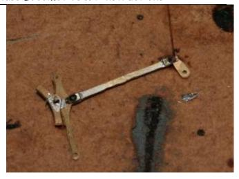
Fold the brake rod (24) 180° and laminated the two halves, this forms a pocket at each end where the rods are mounted to the crank and hangers. Insert a 0.3mm wire through the rear hole and the short crank (29), then thread the crank onto the rear pivot and insert a second piece of 0.3mm wire through the front hole and the rear brake hanger. Solder the wire to the back of the brake rod with resin cored solder, tirm the wire off the back and file the front side back to represent the pins
