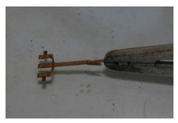
Take the reversing lever (9), punch the rivet details at the handle and rack ends. Fold the lever 180° and solder it back to back, this should leave a rack on either side of the lever and a tiny flat on the bottom. Position the lever on the left hand side between the tank and the boiler, check with the bottom of the lever and align the two halves then solder the lever to the cab floor.
