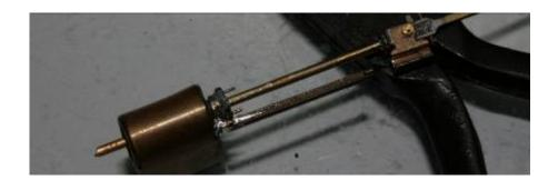
Cut the piston rod to length between the two marks
