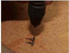
Clean up the steam valve casting, drill out the holes in the nuts to 0.5mm, insert 3 short lengths of 0.5mm wire and solder into each nut, enlarge the hole in the top of the boiler at the half etch location, bend the wire pipes to fit down either side of the boiler and solder in place.
