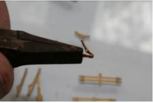
Open out the top mounting hole to 0.5mm and the bottom hole to 0.4mm.
