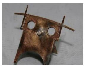
Remove the pressure gauge (30) and fold 180° leaving the tab between the two halves to form the pipe union. Position the gauge in the centre of the base between the windows on the cab front and again with a small amount of solder paste sweat the gauge into place
