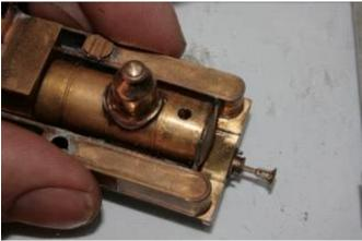
Enlarge the hole in the top of the smoke box and attach the funnel by soldering from the inside of the boiler. Tack solder through the hole and check alignment before soldering completely.
