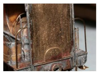
Take a length of 0.5mm wire and bend it to fit from the hand rail hole in the side angle to the hole in the floor. Check both sides are the same and solder in place.
